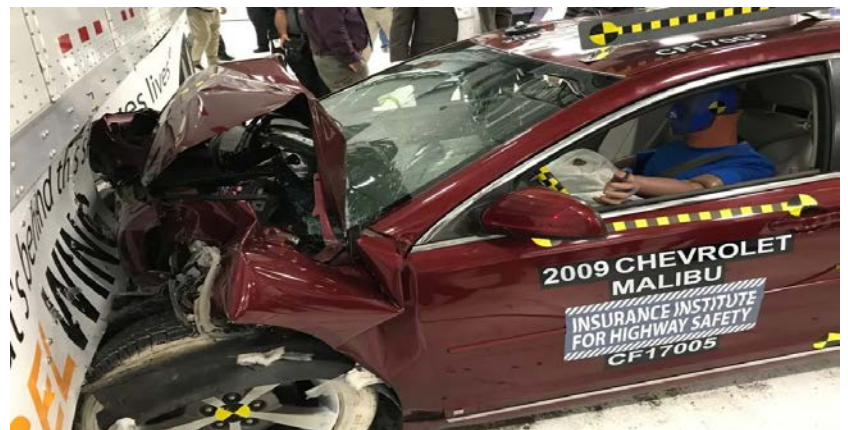
Side Guard Successfully Prevented Passenger Compartment Intrusion
