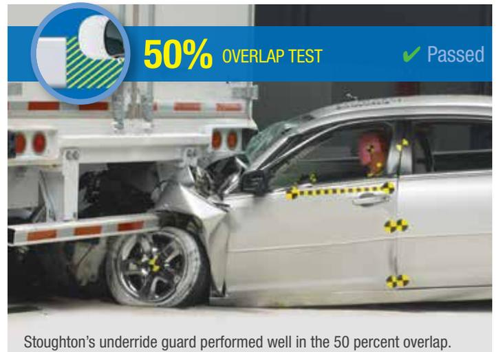
These guards generally work well to prevent underride, except in crashes occurring at the outer edges of trailers, the crash tests show.
