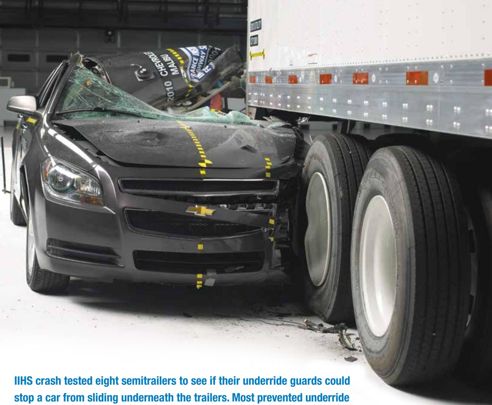
**IIHS crash tested eight semitrailers to see if their underride guards could stop a car from sliding underneath the trailers. Most prevented underride in the two easier tests. Only one trailer passed the toughest test, a 30 percent overlap.**
