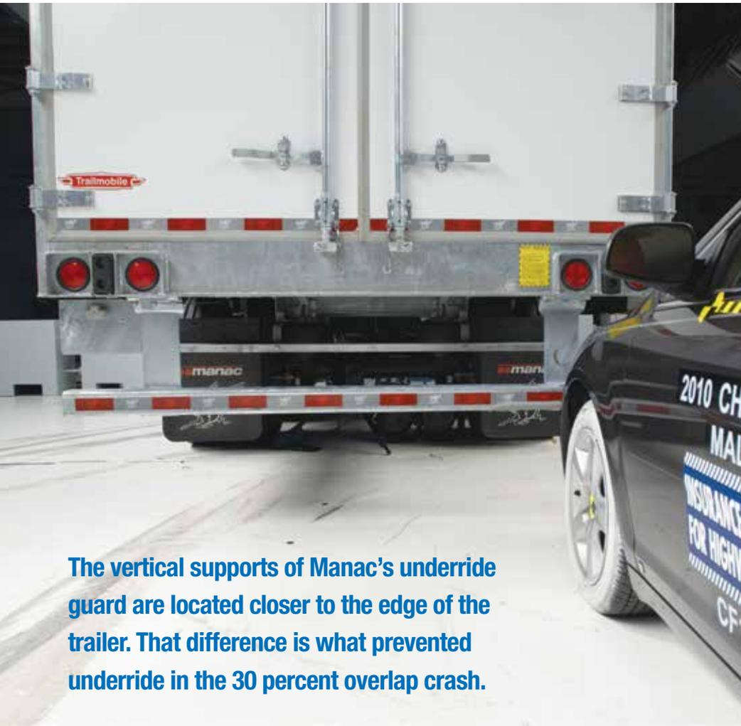
The vertical supports of Manac’s underride guard are located closer to the edge of the trailer. That difference is what prevented underride in the 30 percent overlap crash.
